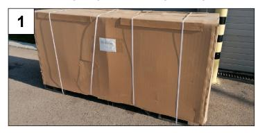
First remove the parcel straps (shown in white on this picture) with a carpet knife. Then remove the cardboard angles (under the parcel straps). Now carefully cut the cardboard open at the side edges. The cardboard can now be carefully removed.
