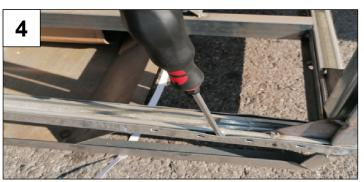
Now flange the subframe to the punched holes using a flat-head screwdriver.
