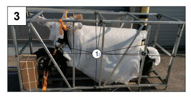
Before you start dismantling the transport scaffold, remove all attachments located in the scaffold. Now locate the hexagon head screws (1) that hold the scaffold together and loosen them.
